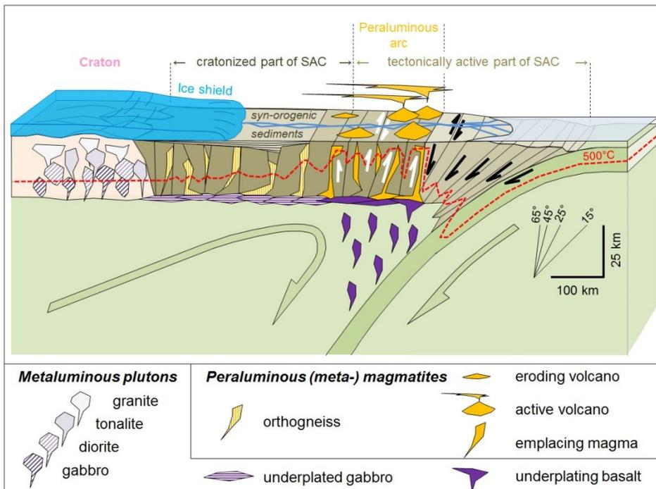
**Fig. 3:** Dynamics of cratonization of a subduction-accretion complex (SAC). The growth of an entire SAC can extend over more than 100 Ma, but the cratonization of a specific part can occur within a short period of c. 10 Ma. (Note that horizontal scale is four times shorter than vertical scale, and structures are virtually steepened in the scheme. The indicated angles are calculated for the shortened scheme.)
